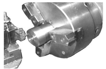
Place the collet facing fixture in the chuck of a lathe so that the threads of the R-8 collet can be faced. This is the end of the collet that will get qualified. Before starting the lathe, touch the facing tool to the front of the fixture and move away .002 so the fixture does not get cut. Now you are ready to cut away any material that may extend beyond the facing fixture.
