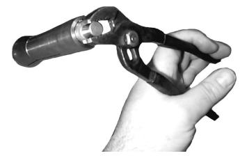
Once you have faced all your collets to length, you're ready to install the pull stud. Clean the collet and pull stud threads so they are free of oil. Next apply loctite thread locker to the pull stud and screw it into the collet. Tighten with pliers and let set.
