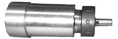
**Example:** if you are facing a ½" collet you should have a ½" pin in the collet. You need to have the corresponding pin with the collet or the collet will not qualify correctly. Once you have secured the collet in place with the correct pin size in the collet you are ready to face the collet to length.
